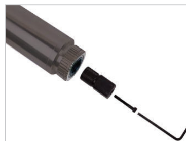
FIGURE 20 – Drive square removal
